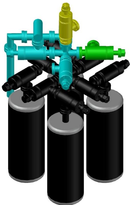
Figure 1. Tank assembly with valves to quadrupole volume (yellow), pumping station (green), and piercing tool (cyan valve at front).
