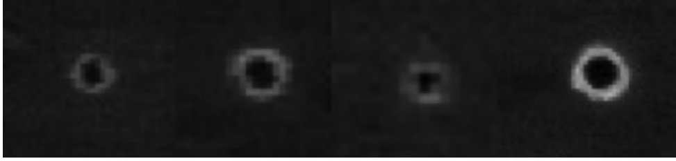
Fig. 2. Secondary electron images of four Stardust cometary craters with diameters (left to right): 500 nm, 500 nm, 250 nm, 750 nm.
