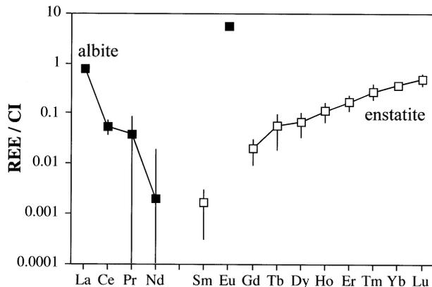
Fig. 2. CI chondrite-normalized REE patterns for albite and enstatite from EET 90102. The enstatite pattern is the average of nine analyses. Elements not shown are below detection limits.
