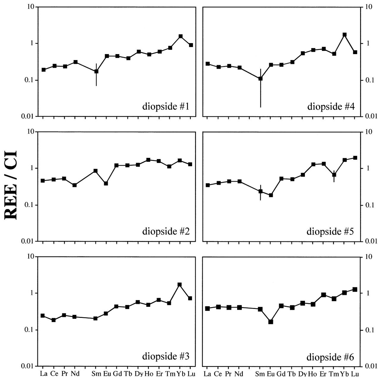
Fig. 3. CI chondrite-normalized REE patterns for diopside from EET 90102. Error bars are shown only for some elements (e.g., Sm, Tm).
