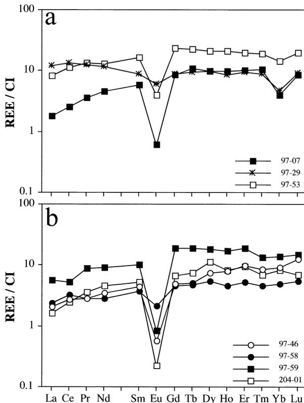
Fig. 5. CI chondrite-normalized REE patterns for diopsides from EH3 chondrites: (a) patterns with Yb anomalies, and (b) patterns without Yb anomalies. The pattern labeled 204-01 is from Qingzhen, the others are from Sahara 97159.
