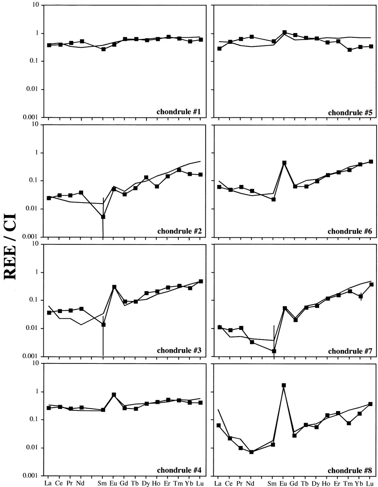
Fig. 4. CI chondrite-normalized REE patterns for relict chondrule fragments from EET 90102. Filled squares show the measured patterns for the chondrules; lines show the results of calculations to reproduce the chondrule compositions from EET 90102 mineral compositions. Error bars are shown only for some elements (e.g., Sm).
