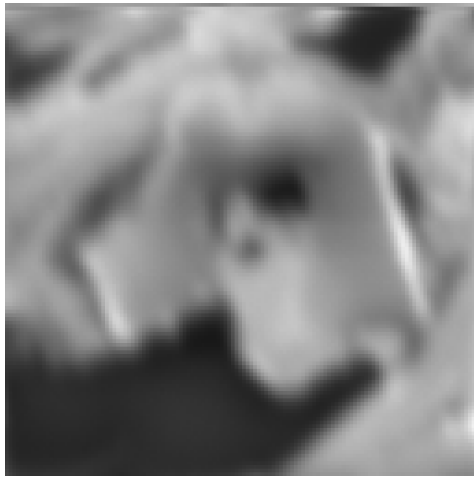
Figure 2: Scanning ion image of ^{16}\text{O} from the spinel grain. Image is 10 \times 10\ \mu\text{m} .
