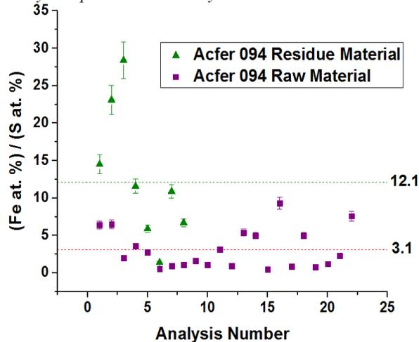
**Figure 3:** Comparison of Fe to S ratios observed in Acfer 094 analog melt layers and those seen in Fe-rich unfired Acfer 094 material. All residue material came from craters 1-3  $\mu\text{m}$  in size. The average Fe/S value of the Acfer 094 residue material (12.1) is nearly four times larger than that of the unfired component (3.1).
