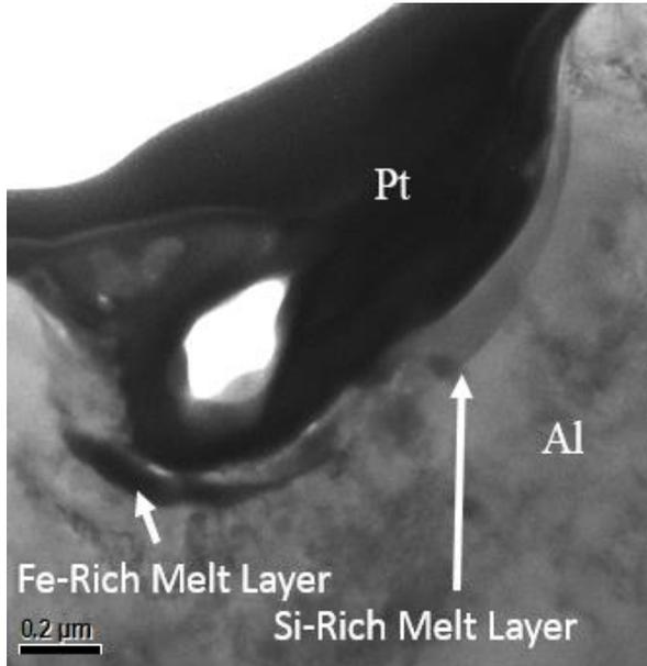
**Figure 2:** TEM image showing the cross section of a 1.4  $\mu\text{m}$  Acfer 094 analog crater. Both darker Fe-rich and lighter Si-rich melt layers are visible between the Pt cap and the Al foil. Al melt from the foil is the primary component in both layers.
