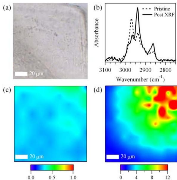
**Figure 2.** (a) Optical image of I1017,6,20 keystone with the space-exposed surface at the top of the image. (b) FTIR spectra before and after S-XRF analysis at ESRF ID13. Image map corresponding to the  $\text{CH}_2/\text{CH}_3$  area ratio (c) prior to any synchrotron X-ray analysis and (d) after S-XRF analysis on ESRF ID13. Note change in color scale.
