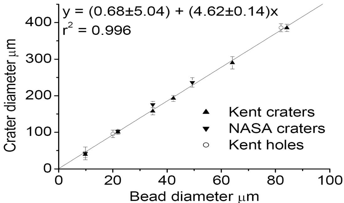
Figure 1: Projectile size versus crater diameter, measured from rim crest to rim crest, in soft aluminum 1100 foils. The open symbols relate to free-standing foils.
